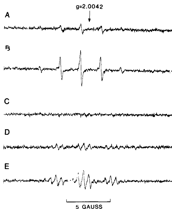
Fig.3. ESR spectra of the semiquinone anion radicals generated by reaction of quinones with glycine or N -acetylcysteine. Reactions contained: A, BQ (1 mM) and glycine (250 \mu M); B, BQ (1 mM) and glycine (20 mM); C, 1,4-NQ (1 mM) and glycine (250 \mu M); D, 1,4-NQ (1 mM) and glycine (20 mM); E, 1,4-NQ (1 mM) and N -acetylcysteine (250 \mu M). The results shown are from one experiment typical of three.
